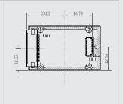
37.00 mm W x 23.40 mm D x 12.00 mm H 38.85 mm W x 23.50 mm x 5.20 mm H (Narrow board with one mounting area and connected by molex cable. The engine is separated.)
